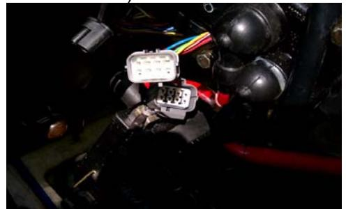
4. Disconnect the Main Relay connector and connect the Early Relay Bypass cable in line between the two halves of the Main Relay connector. Fasten the ring terminal of the Early Relay Bypass cable to the negative/ground (-) post of the battery.
