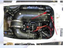
2.6 (Below) Remove the two 12mm bolts securing the stinger pipe to the cylinders. Remove the two 12mm bolts from the stinger piep brace. Wiggle the pipe towards the front of the boat and pull it up and out of the hull.
