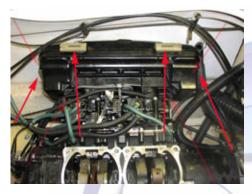
3.2 (Below) Remove the four 10mm bolts holding the intake cover base to the carbs. Remove the intake cover base.
