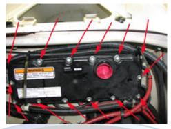
4.11 (Below) Unscrew the two ground cable screws and disconnect the quick connects. Remove the cable from the box.
