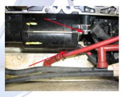
4.6 (Below) Pull the two rubber PTO shroud mounts out and slide the PTO shroud forward and remove it from the hull.
