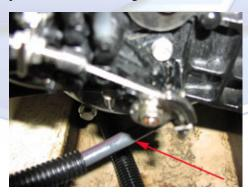
4.4 (Below) Disconnect the oil return line from the oil tank.
