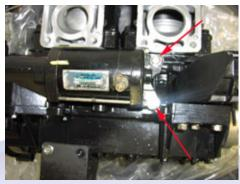
5.8 (Below) Remove the eight 12mm bolts from the exhaust manifold.
