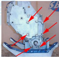
3.7 (Above) Remove the six 10mm bolts securing the exhaust bracket to the engine and remove the bracket.
