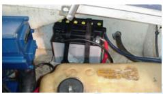
1.1 (Above) Remove the two retaining straps, disconnect the battery and remove it from the hull. Disconnect the negative (black) cable first, then the positive (red).
