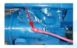
2.7 (Below) Remove the four motor mount bolts with a 12mm socket (carb side shown).
