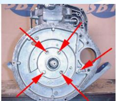
3.18 (Below) Remove the equalization lines from the block.
