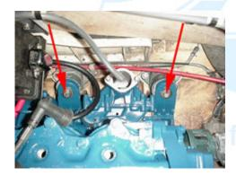
2.8 (Below) Remove the PTO coupler shield with a 10mm socket.
