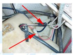
2.10 (Below) Remove the three 10mm bolts and remove the electrical box from the hull.
