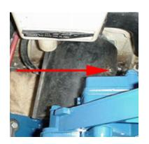
2.9 (Below) Detach the starter switch electrical harnesses.
