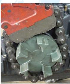
3.5 (Above) Using a chain wrench, remove the PTO coupler.
