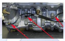
6.2 (Below) Remove the water line to the case cooler. Remove the twelve 10mm flywheel cover bolts, remove the flywheel cover.
