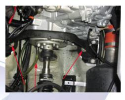
5.6 Lift the front of the engine and slide it backward disengaging the driveshaft from the PTO.
