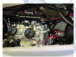
3.3 (Below) Loosen the hose clamp to the air line on the fuel rail and remove the line. Swing the fuel rail over the side of the hull and leave it there for engine installation.
