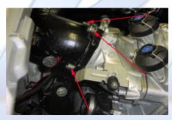
4.8 (Below) Wiggle the exhaust straight up away from the exhaust manifold and loosen the hose clamp to the water hose. Remove the hose.
