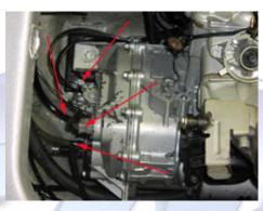
5.4 (Below) Remove the 13mm bolt securing the engine to the front engine mount. Remove the two 13mm bolts securing the engine mount to the hull and remove it from the hull.
