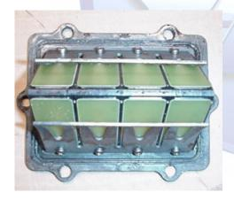
6.7 (Below) Look at each petal-to-cage surface and check for gap. If a gap of more than 0.015" is present, replace the petals.
