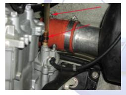
4.5 (Below) Remove the two water lines to the top of the pipe.
