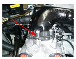
3.5 (B elow) U sing an 8mm Allen wrench and 15mm wrench or Sea-Doo Special Tool 529 035 505, rem ove the three bolts and one nut from the pipe at the manifold.
