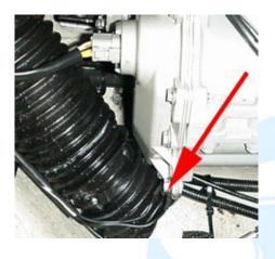
4.4 (Below) Remove the block ground and starter positive wire with a 10mm socket.
