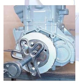
5.14 (Below) Remove the bendix support plate with an Allen wrench.
