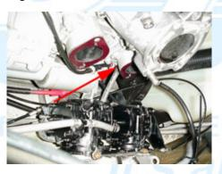
2.8 (Below) Remove the head cooling line, thermo sensor and spark plugs.
