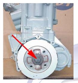
5.13 (Below) Using a universal flywheel puller, remove the PTO flywheel.
