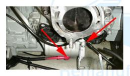
4.5 (Below) Remove the case cooling line from the engine.
