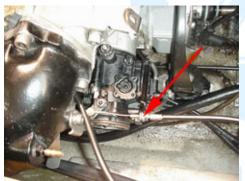
2.6 (B elow) L oosen t he f our 6m m Al len bolts to remove the carbs with a ball Allen socket, if you have one. Remove the Allen bolt securing the carb bracket to the pipe.
