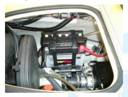
1.1 ( Above) Remove t he two ret aining straps, disconnect the battery and remove it from the hull (XP sh own). Disconnect the negative (black) ca ble first, then the positive (red).
