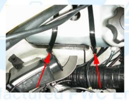
2.2 (B elow) R emove the two 10mm bol ts securing the intake flaps to the brackets. Remove the flaps. Pull the intake snorkels up and out of the hull.
