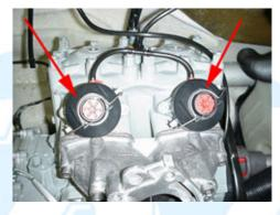
4.7 (Below) Detach the vacuum lines from the R.A.V.E. housings.
