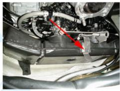
2.4 (Below) Loosen the gast ank captorelieve pressure. Be sure the fuel switch is turned to the "OFF" position, and be aware of any fuel that may spill from the hoses. Make sure the hull is cleared of any gasoline fumes before continuing work, especially with power tools.
