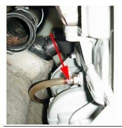
4.6 (B elow) Remove the R.A.V.E. val ve caps by pu shing the retaining clips back. Lift the caps and the springs out. R emove the pulse line at the case that runs to the RAVE valves.
