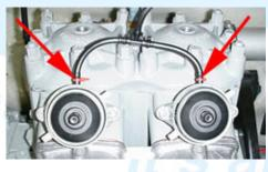
4.8 (Below) Using a 12mm socket, remove the front motor mount bolt. Also remove the two 12mm bolts securing the mount to the hull and slide the mount out of the hull.
