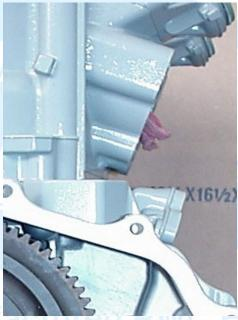
5.9 (Below) Using a 10mm socket, remove the 1 2 b olts fr om t he fl ywheel housing cover a nd r emove i t. It i s SB T's recommendation that t he oil pum p be removed from the new engine, and a block-off plate be installed at this time.
