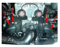
2.3 (Below) Bend the clip up on the flame arrestor to detach it. Slid e it o ff the carburetors and move it forward in the hull to remove it.
