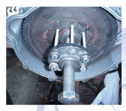
5.11 (Below) Remove the ten 13mm bolts securing the flywheel housing to the block, and remove it. Tap out the front oil seal replace and
