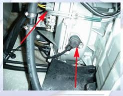
4.2 (Below) Remove the two cooling lines on the flywheel cover
