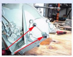
4.3 (Below) Remove the ground cable from the case using a 12mm socket.
