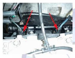
4.8 (Below) Remove the cooling line and air intake line.
