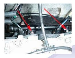
5.5 (Below) Remove the two 14mm bolts securing the head pipe support to the case. Remove the support.
