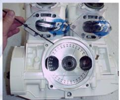
(Below) Place a screwdriver, or use a TDC gauge in the front (MAG) cylinder through the spark plug hole. Turn the crankshaft to find Top Dead Center of this piston.
