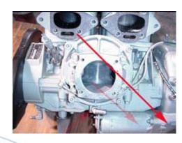
5.9 Remove 3 of the 6 bolts holding the magnet cup to the flywheel (every other bolt, not 3 in a row). **DO NOT REMOVE THE MAGNET CUP FROM THE FLYWHEEL; IT IS TIMED TO ITS LOCATION.** Use a 27mm socket and remove the nut holding the flywheel to the crankshaft.
