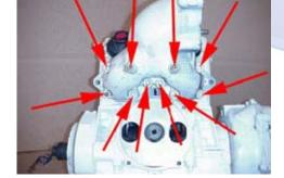
5.5 (Above) Remove the 10 8mm Allen bolts and the exhaust manifold.
