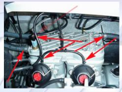
2.2 (Below) Remove the air silencer cover by sliding the 6 tabs off and pulling the cover up and out.
