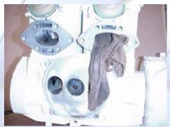
5.8 (Below) Remove the three allen head bolts securing the starter. Remove the Starter.
