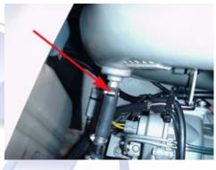
3.3 (Below) Remove the 13mm bolt from the header pipe, and the two 13mm bolts securing the brace to the flywheel housing. Remove the brace. Disconnect the water line from the header pipe.
