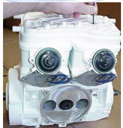
(Below) Align the rotary valve as shown, so that the port is open, and the edge of the valve matches as precisely as possible with the mark. NOTE: the valve is asymmetrical. Flip it around to find the closest match.
