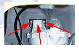
4.6 (Below) Remove the starter wire with a 10mm socket.
