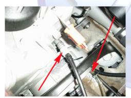
4.9 (Below) Remove the two rear engine mount bolts with a 13mm socket. Loosen the clamp around the driveshaft at the PTO and slide the engine approximately 4" forward to clear the driveshaft. NOTE: There are two rubber bumpers on either end of the driveshaft. Make sure you don't lose them, and make sure to replace them, if removed. If possible, have someone hold the driveshaft while you slide the engine to prevent the impeller side bumper from disengaging. Lift the engine out of the hull.
