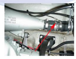
3.2 (Below) Disconnect the waterlines coming from the pipe and from the head. Remove the clamp by loosening it with a screw driver.
