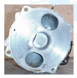
Examine the rotary valve itself. It must also be free of any imperfections. It must not have any pitting, holes, scratches, dings, dents, bends, etc. If any of these are present you MUST replace the valve. We recommend the use of ONLY OEM valves.
