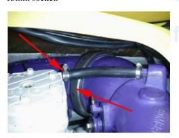
3.3 (Below) Remove the 13mm bolt from the header pipe, and the two 13mm bolts securing the brace to the flywheel housing. Remove the brace.
