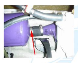
3.2 (Below) Disconnect the waterlines coming from the pipe and from the head. Remove the clamp by loosening it with a 13mm socket.
