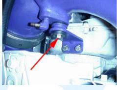
3.4 (Below) Remove the three 8mm Allen bolts and one 17mm nut from the exhaust header pipe. Loosen and remove the head pipe.
