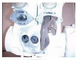
5.7 (Above) Stuff a rag into one of the exhaust ports. Make sure the rag penetrates through the port, into the combustion chamber on top of the piston. This will prevent the engine from turning over while you remove the flywheel nut & PTO coupler.
