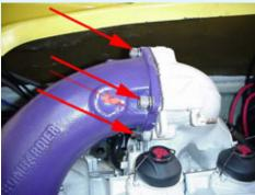
3.5 (Below) Remove the two 8mm Allen bolts securing the stinger pipe to the block. Remove the stinger pipe by moving the front electrical box out of the way, and sliding the pipe forward through and out the front hood cavity. Remove the two water lines on the T-fitting, found under the stinger pipe mounting point.
