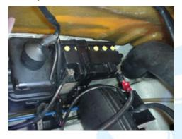
1.1 (Above) Remove the two retaining straps, disconnect the battery and remove it from the hull. Disconnect the negative (black) cable first, then the positive (red).
