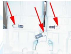
5.3 (Below) Remove the five 13mm bolts from the engine support and remove it.
