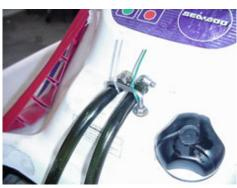
2.8 (Below) Loosen the gas tank cap to relieve pressure. Disconnect the fuel supply and return lines. Be sure the fuel switch is turned to the "OFF" position, and be aware of any fuel that may spill from the hoses. Make sure the hull is clear of any gasoline fumes before continuing work, especially with power tools.
