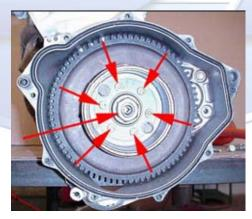
5.9 Install a universal flywheel puller into the exposed threaded holes in the magneto cup and remove assembly.
