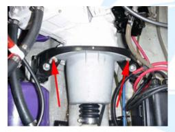
4.3 (Below) Remove the front engine mount bolt and two bolts securing the mount to the hull with a 13mm socket.
