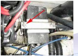
1.1 (Above) Loosen the front retaining wing nut, swing the retainer plate back and remove the plastic protective cover.
