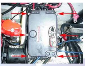
5.3 (Above) Open the electrical box by removing the six bolts with an Allen wrench.
