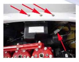
4.3 (Below) Loosen the two clamps using a 10mm wrench. Remove the two 13mm bolts holding the exhaust pipe to the exhaust manifold. Pull the exhaust pipe straight back and remove it from the hull.
