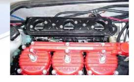
3.4 (Below, Right) Remove the throttle, oil pump and choke cables from the carburetor assembly. Pivot the shafts for easy removal of the cable endbarrels.
