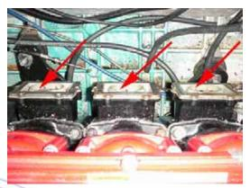
3.8 (Above) The intake manifold is fastened with 18 bolts; 6 per intake tract. The bottom 6 bolts are hidden in the picture but are inline with the top bolts. Remove them all with a 10mm socket.
