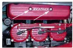
3.2 (Above) Remove the flame arrestor cover bolts with a 13mm socket.
