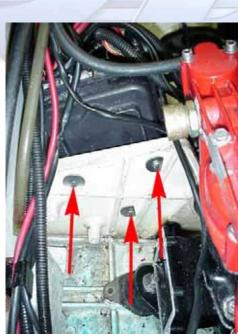
5.4 (Right) NOTE: DO NOT CUT THE WIRES! Disconnect all wires coming the through the grommet into the box. Note the location of the wires connected directly to the circuit board for later installation. All other wires are color coded. Remove the two Allen head bolts & grommet from the box then pull the wires through and out.
