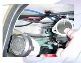
3.5 (Below) Loosen the gas tank cap to relieve pressure. Remove the front carb fuel-in and pulse lines from the assembly. Loosen the hose clamps with a screwdriver and gently twist off the hoses. Be sure the fuel switch is turned to the "OFF" position, and be aware of any fuel that may spill
