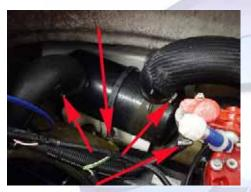
(For those engines with 4.2 (Below) electric reverse.) Remove the three 5mm allen head bolts holding the electric reverse in place. Disconnect the quick connect and slide the box toward the back of the hull and set it in the footwell.
