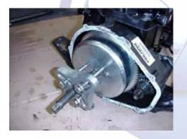
6.5 (Above) Remove the end nut on the shaft with a 19mm socket. The rag in the exhaust port for PTO coupler removal will again prevent the engine from turning over, allowing the nut to be removed. Next use a universal flywheel puller to remove the flywheel from the shaft. **CAUTION:** Do not screw the puller screws into the flywheel more than 5 complete turns or damage to the stator may occur.
