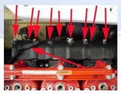
4.5 (Below) After removing the exhaust manifold from the hull, remove the block ground bolt and the starter wire nut & washer using a 10mm socket.
