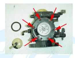
1.4 (Below) Remove the check valve diaphragm.
