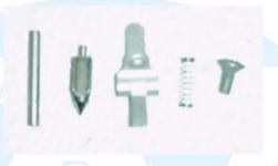
2.6 (Below) Inspect the needle and seat. The needle should have a smooth edge with no signs of grooving or wear. If present, replace the needle and seat combo. Inspect the seat internally for signs of corrosion and sediments. It should have a polished brass appearance. If not, take a small piece of sand paper, roll it into a small tube and sand the inside clean. Rinse with carb
