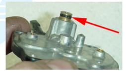
1.7 (Below) Remove the o-ring from the circuit chamber. Remove the two screws securing the high-speed circuit to the chamber and remove the plate. Remove the gaskets and film-valve.
