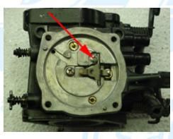
1.5 (Below) Remove the center screw holding the regulator chamber to the carb and remove it. Remove the fuel filter.
