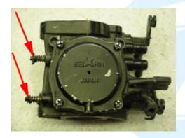
1.2 (Below) Remove the four screws from the regulator chamber cover and remove it.
