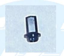
2.5 (Below) Inspect the needle and seat. The needle should have a smooth edge with no signs of grooving or wear. If present, replace the needle. Inspect the seat internally for signs of corrosion and sediments. It should have a polished brass appearance. If not, take a small piece of sand paper, roll it into a small tube and sand the inside clean. Rinse with carb cleaner.
