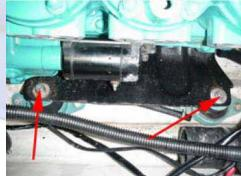
4.5 (Below) Remove the two 10mm bolts from the electrical box to expose the wiring harnesses beneath. Detach the wiring harnesses. **NOTE: DO NOT CUT THE WIRES!** Remove the engine from the hull.
