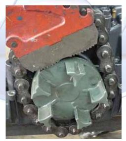
5.5 (Below) Remove the seven 10mm bolts securing the flywheel cover to the engine and remove the cover.
