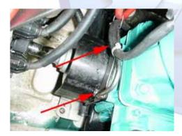
4.3 (Below) Remove the two PTO cover studs with a 6mm stud socket.
