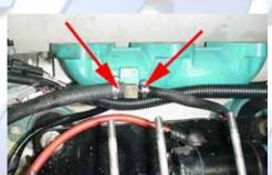
3.5 (Below) Remove the nine exhaust studs with an 8mm stud socket. Remove the starter ground and positive wires with a 10mm socket.
