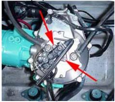
4.2 (Below) Remove the two 10mm nuts securing the PTO cover to the engine and remove the cover.
