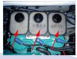
2.3 (Below) Remove the six 10mm bolts securing the flame arrestor base and carbs to the manifold and remove the base.
