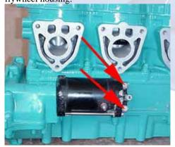
5.3 (Below) Stuff a rag into an open exhaust port. This will prevent the engine from turning over while removing the flywheel and PTO coupler.
