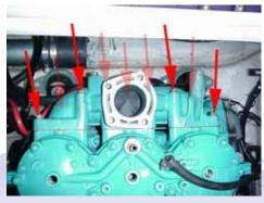
3.4 (Below) Disconnect the water lines from the manifold. Remove it from the hull.
