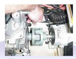
Take a small straight edge and place it on the coupler. You are looking for an even match all the way around the coupler. Place shims where necessary to align the couplers.
