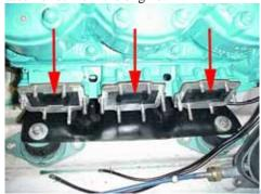
2.7 (Below) Inspect each reed assembly for damage and wear. Look at each reed petal and inspect the edges for signs of cracking, chipping or any missing parts. If any damage is present, replace the petals.
