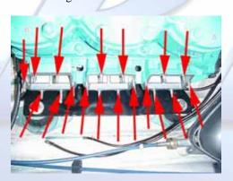
2.10 (Below) Remove the throttle and choke cables from the bracket, then remove the two 10mm bolts securing the bracket to the cylinder and remove it.
