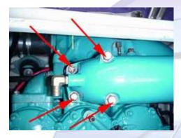
3.3 (Below) Remove the nine 12mm nuts securing the exhaust manifold to the engine and pull the manifold back off the studs.
