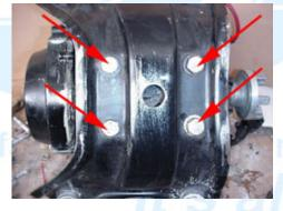
4.10 (Below) Tap the nut retaining tabs back to gain access to the nut. Remove the flywheel nut with a 19mm socket.
