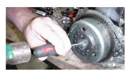
4.12 (Above) Using a chain wrench, remove the PTO coupler.
