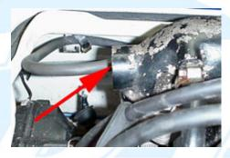
2.3 (Below) Remove the four 10mm nuts / bolts from the exhaust manifold and bracket. Remove the exhaust pipe from the hull.
