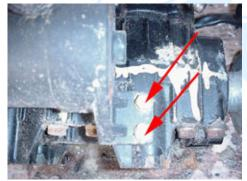
4.7 (Above) Remove the two 10mm bolts securing the starter motor. Pull the starter motor firmly back and out of the flywheel housing.
